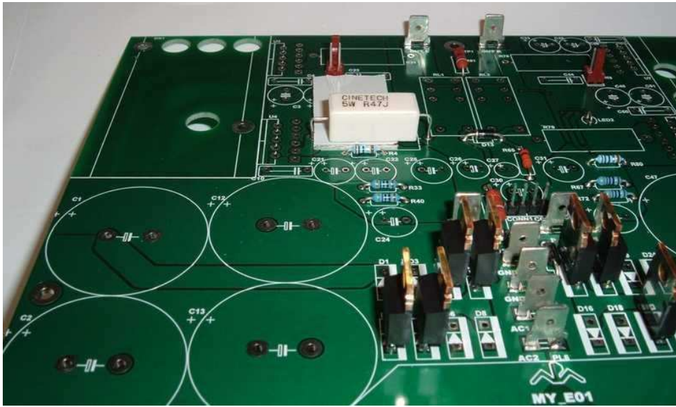
Fig4 Mounting detail of diodes and power resistors
