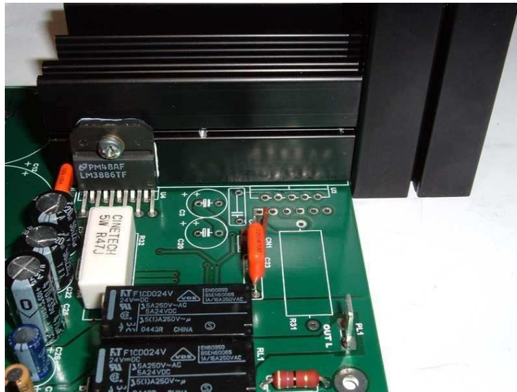
Fig8 verify the PCB-headsink (lateral) alignment
