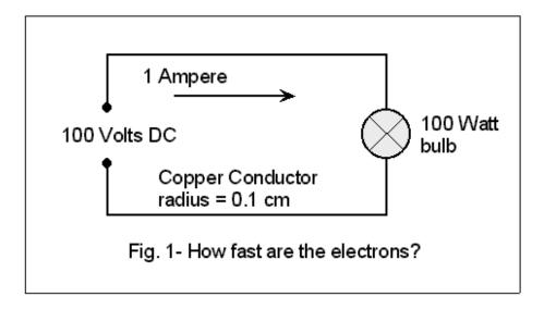
We will use a light bulb of 100 watts. To simplify the maths a little we will say the bulb operates at 100 Volts. The current the bulb will draw will be 1 ampere for 100 watts; from P=ExI, therefore I=P/E.
