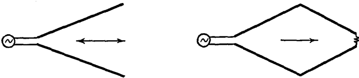
FIG. 35 I. "V" and Rhombic types of antenna
