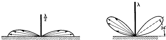
FIG. 8 E. Radiation patterns from vertical Marconi antennas
