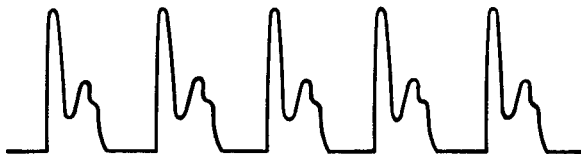
Fig. 95. Anode current with shunt-tuned filter.
