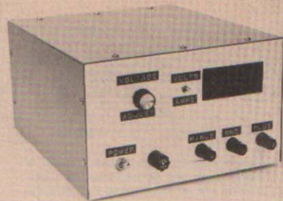
Fig. 37. — Front view of the deluxe 5- to 25-volt, 5-ampere power supply.
