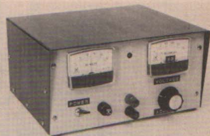
Fig. 34 — Front view of the 0-to 25-volt, 1.5-ampere power supply.
